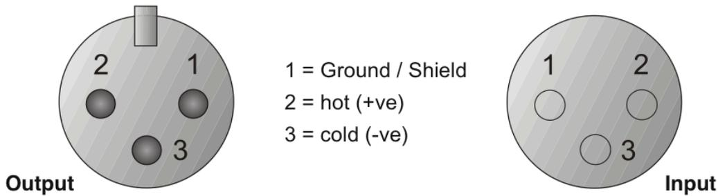
For unbalanced use PIN 1 and PIN 3 have to be bridged
